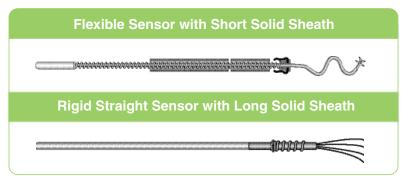
Figure 2. Flexible temperature sensors, like the WORM have a minimized solid sheath. (In the case of the WORM, only 1.5 inches.) This shorter solid sheath leads to step response times 13 percent faster than standard straight sensors.
