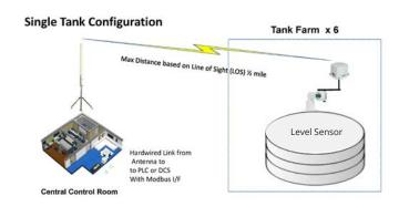
Shown is a single tank configuration outlining how the Sentinel node interfaces with the level sensor in transmitting data to a Gateway that ties into a PLC within a central control room. All transmission distances are based on good line of sight.
